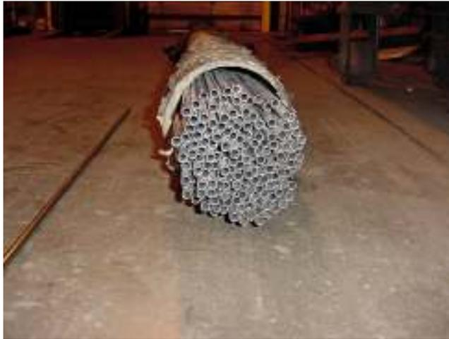
Figure 13. 0.405" OD X .035 wall X 7' long 304 stainless steel, vacuum soft annealed tube sleeves.
