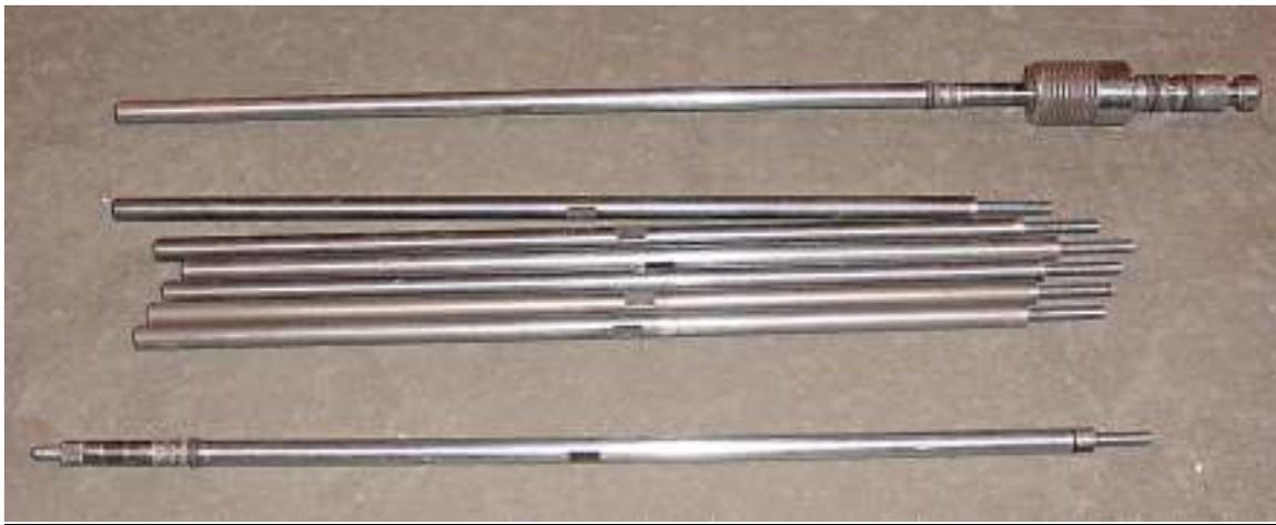
Figure 14. Hydraulic Expansion Mandrels designed to fit into the 7E and 7W heaters confined space.
